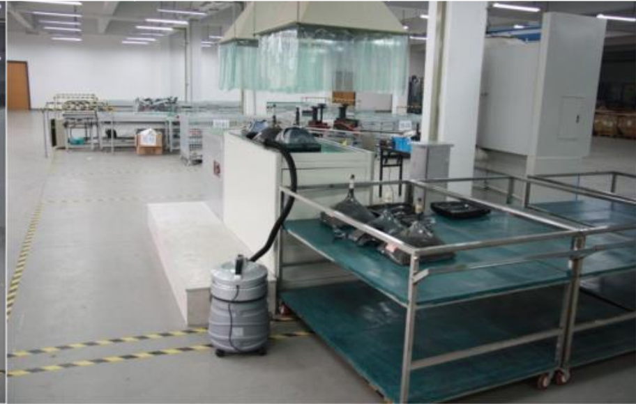
Separating the funnel and panel glass
