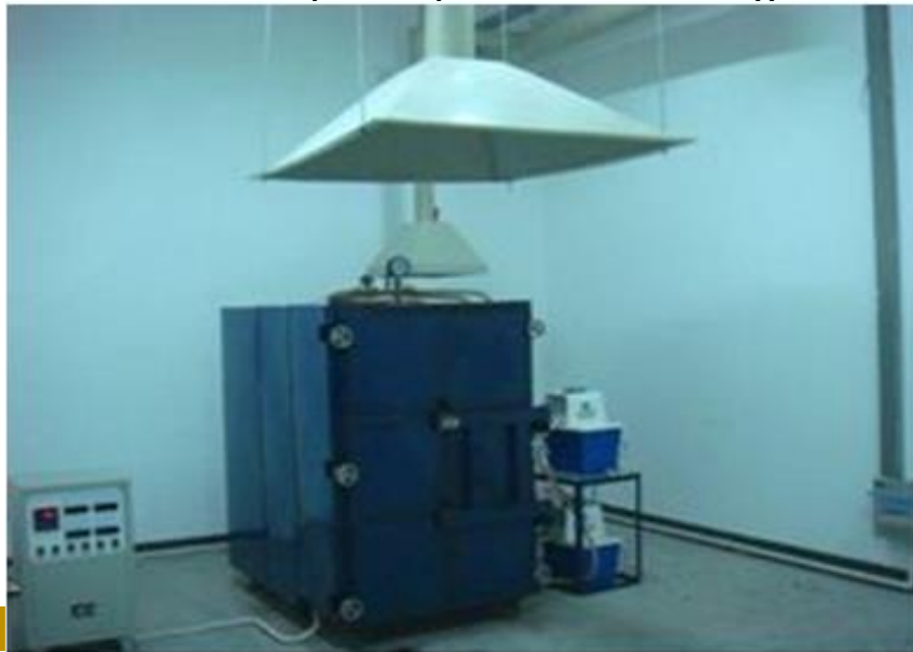
Furnace for LCD and thermal shock treatment of PCBs
